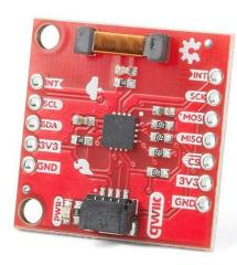
Add the <u>SparkFun Qwiic Lightning Detector</u> to your next weather station to make sure you're aware of any potential hazards heading your way. The AS3935 is capable of detecting lightning up to 40 km away, with an accuracy of 1 km to the storm front, and has a sensitive antenna tuned to pick up lightning events in the 500 kHz band.
